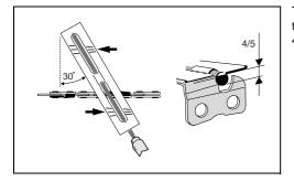
The file holder makes file guidance easier. It is marked for the correct 30° sharpening angle (keep the marks parallel with the chain when filing, see illustration) and limits the cut depth to the correct 4/5 of the file diameter.
